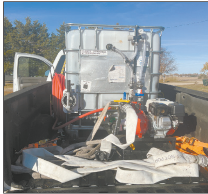
These pictures were taken after the unit was used at a burn and the hoses were thrown back in the pickup. The garden hose is on a hanger and the 1" when under pressure lays beside the unit so it's not as messy as it looks in the photo. The 2" hose can't be used unless all 25' is strung out.
